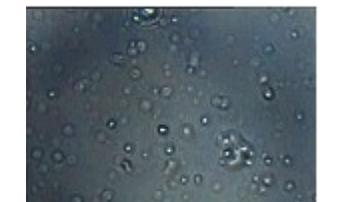
Pic. 4: After 60min of fine grinding: 2-3micron
